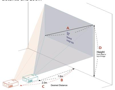
The table below shows how to achieve a desired image size by adjusting either the position or the zoom ring. For example: to obtain an image size of 50" set the projector at a distance 1.6 m and 2.0 m from the screen and adjust the zoom level accordingly.
